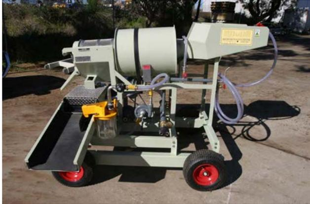
Professionally built in WA. 2 tph. Large capacity scrubber for the treatment of high clay content material. Twin fines concentrators, Tails sluice. Fines sluice. Engine plant powered by a Honda GX 200. Mounted on wheels but can be put on a trailer.
